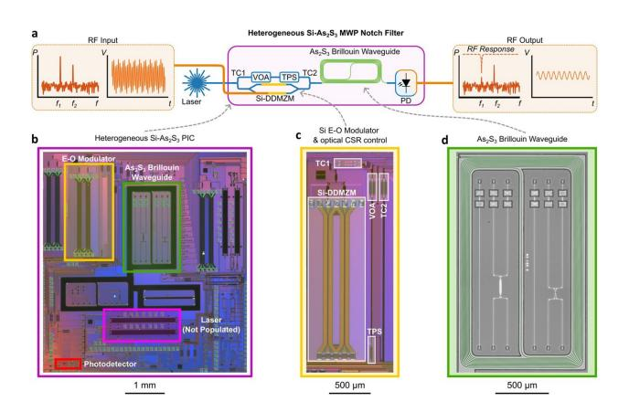
Heterogeneous integration of  $As_2S_3$  waveguides and silicon components for an on-chip microwave photonic filter system. Credit: *Nature Communications* (2023). DOI: 10.1038/s41467-023-43404-x
